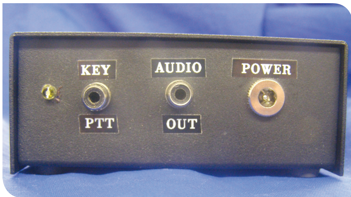
Decoder located at the rig. Key/PTT connects to PTT jack on the rig.
