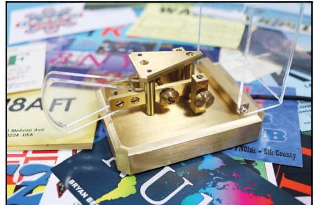
My Schurr PROFI-2 "rescue" keyer. Both acrylic paddles snapped off at the joint and were repaired with just a touch of WeldOn 4.
